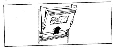
**To replace door:** Grasp the door at each side, align slots in the door with the hinge arms and slide the door down onto the hinge arms until it is completely seated on hinges.
