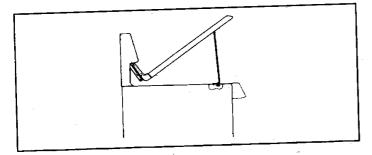
**To lower the top:** Hold the front edge of the cooktop and carefully push back on each support rod to release the notched support. Then gently lower the top into place. The support rods will slide into the range frame.
