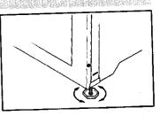
range should be secured to the floor by sliding a rear leveling leg into the anti-tip bracket supplied with the range.
