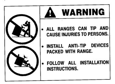
**WARNING:** To reduce the risk of tipping of the appliance from abnormal usage or by excessive loading of the oven door, the appliance must be secured by a properly installed anti-tip device.
